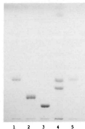
Fig. 10. HPTLC of porcine and human brain GM1 fractions. The plate was developed in chloroform-methanol-0.2% CaCl 2 60:35:8 and gangliosides were detected with diphenylamine reagent spray. Lane 1: authentic GM1; lane 2: authentic GD1a; lane 3: authentic GD1b; lane 4: porcine brain GM1 fraction (containing fucosyl GM1); lane 5: human brain GM1 fraction.
